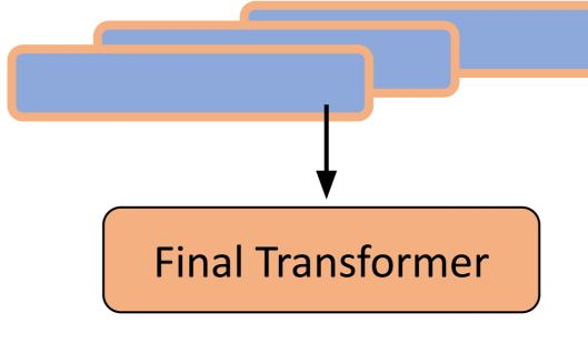
2<sup>nd</sup> stage: the entire sequence is encoded, by computing attention between its rows.
